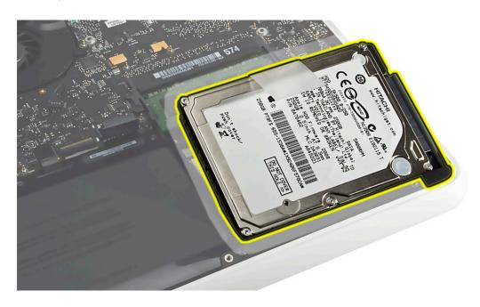
**9** Disconnect hard drive connector cable.
